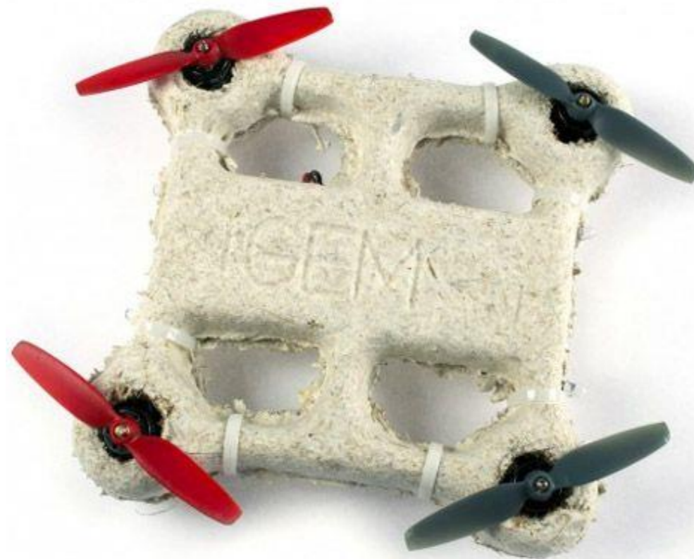
14- the GEM modular, biodegradable drone. Image sourced from: www.washingtonpost.com/news/speaking-of-science/wp/2014/11/22
