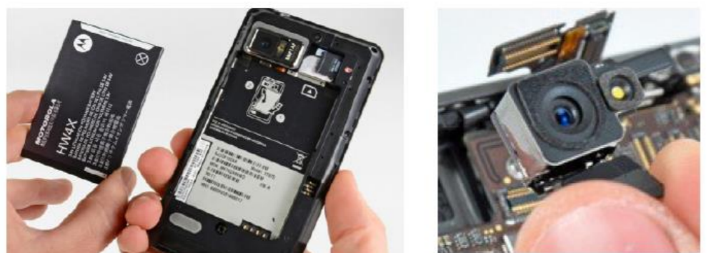
9- Overview of alternative joining techniques in electronic devices for (from left-to-right) a display assembly in an iPad joined to the body using snap fits, LCD screen in a Motorola phone is disassembled using snap fits, memory chips clicked into the motherboard of a desktop computer, CPU clicked onto the motherboard of an HP computer, non-integrated battery in a Motorola phone and a camera clicked onto a motherboard in a mobile phone (source: Floras CEIP report Designing for a Circular Economy , iFixit & HP)
