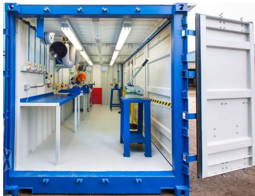
27- A company called Mr-Box already specialise in converting old shipping containers into mobile workshops. Image sourced from: www.mrbox.co.uk/container-gallery/opensided-containerised-workshops/
