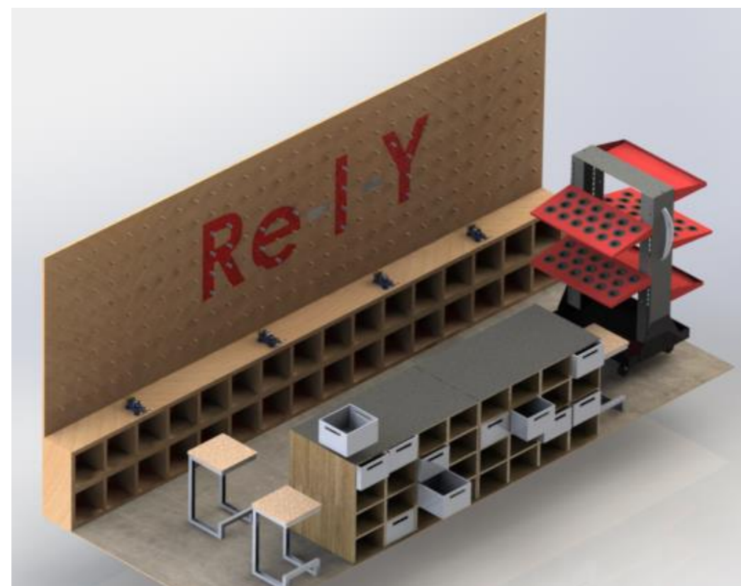
20- A CAD model of a possible mobile Re-I-Y unit in a 2400mm x 6100mm shipping containers, created on Solidworks
