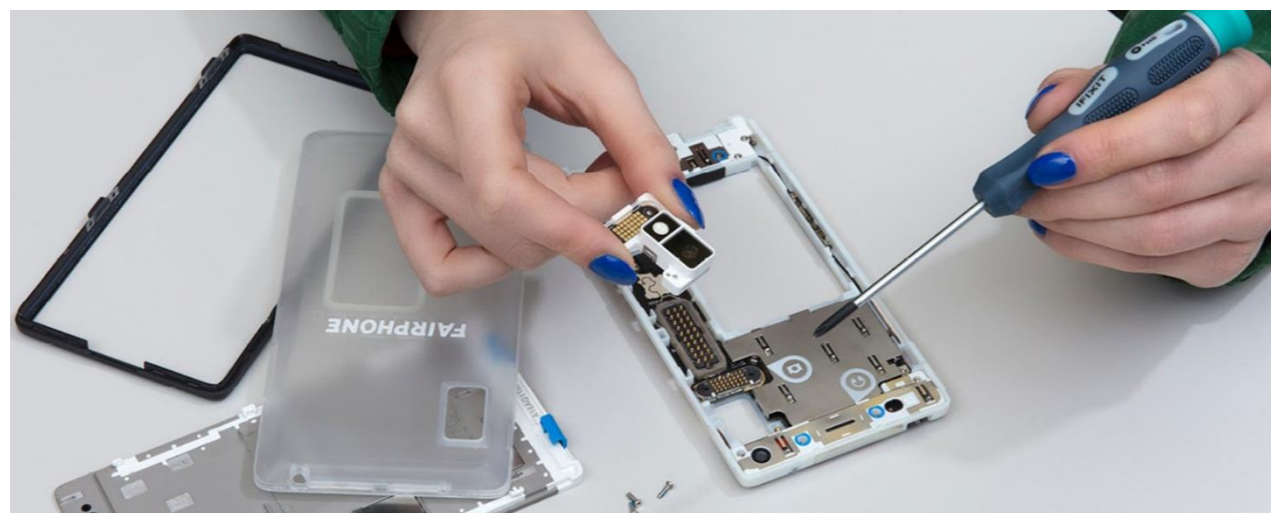
16- A user easily replaces the modular camera in a 'Fair Phone', image sourced from: https://www.ellenmacarthurfoundation.org/explore/circular-design
